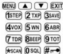
Figure 2.3. BTECH GMRS-V1, keypad
